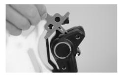
Prepare the front wheel: remove the brake pad spacer.
