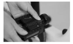
Screw the pedal onto the connecting rod thread with your hand, giving two or three turns. Clockwise. It is recommended to use mounting paste.
