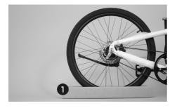
Take out the frame, which has the front wheel and the handlebar are fixed to it. Use the packaging cartons ① to hold the bike.
