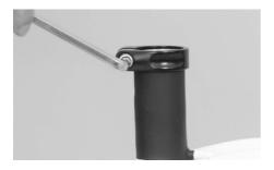
Unscrew the fixing screw of the seat post clamp with the 6 mm Allen key.
