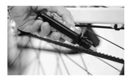
In isolated cases you may need Teflon oil inside the teeth. Apply it and clean the excess.
